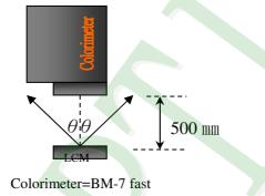
To be measured at the center area of panel with a viewing cone of 1° by Topcon luminance meter BM-7, after 10 minutes operation (module)
