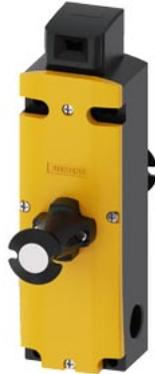
Safety position switch with tumbler Locking force 1300 N 5 directions of approaches Spring-locked Emergency release at the rear and Escape release on the front Magnet voltage 24 V DC Monitoring actuator 2 NC/1 NO Monitoring magnet 2 NC/1 NO Supplied without actuator. Actuator 3SE5000-0AV0. please order separately
