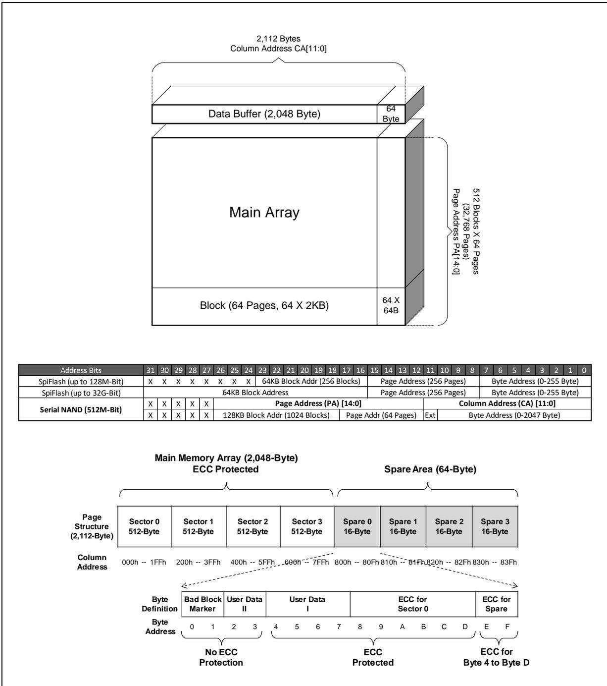
Figure 2. W25N512GV Flash Memory Architecture and Addressing
