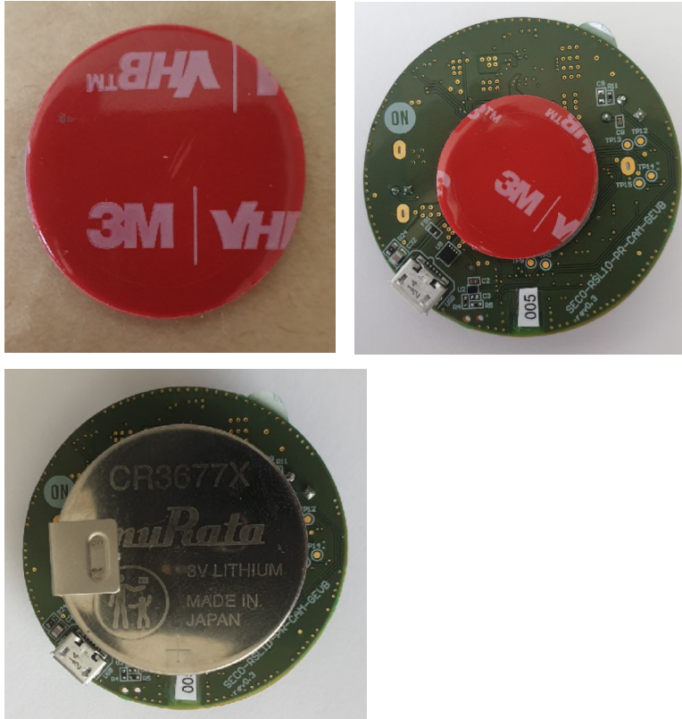
Figure 6. Process of Attaching the Sticker onto the Bottom Side of the PCB and Battery Insertion
