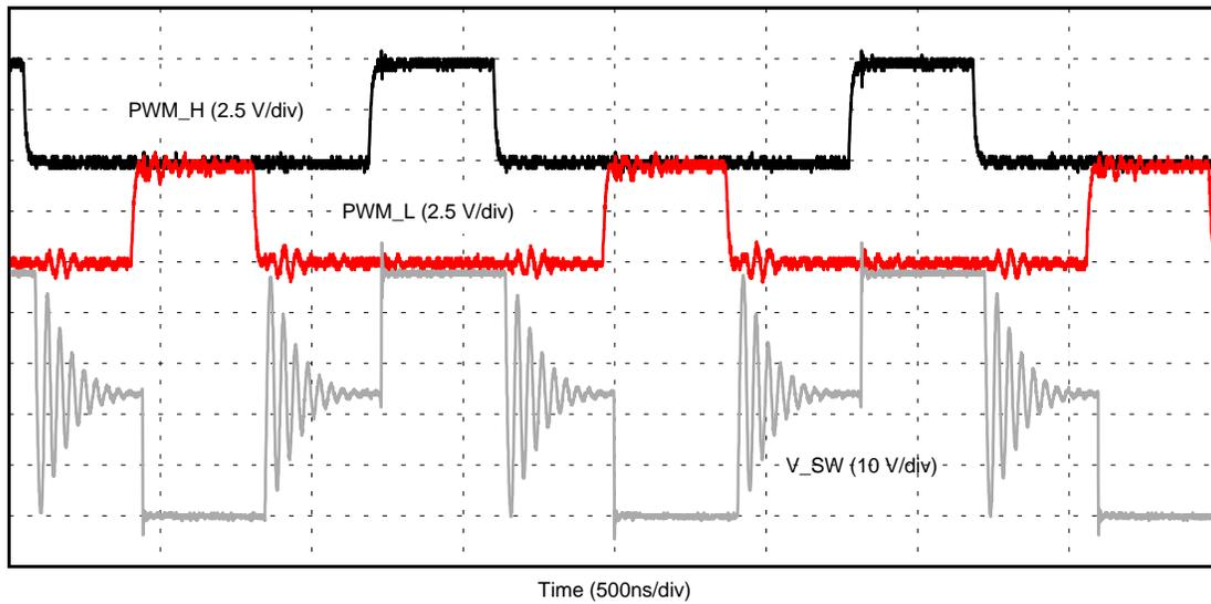
Figure 7. Primary-Side Switching Waveforms
