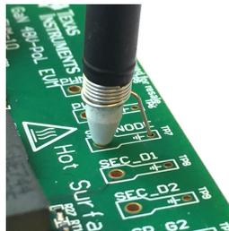
**Figure 5. Recommended Probe Usage for Test Points**
