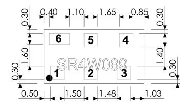
1-5 copper pads: 1.0 x 1.0 (mm) 6 copper pad: 1.5 x 0.8 (mm)
