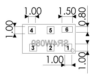
1-5 copper pads: 1.0 x 1.0 (mm) 6 copper pad: 1.5 x 0.8 (mm)
