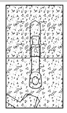
3.) Hammer the anchor into the hole.
