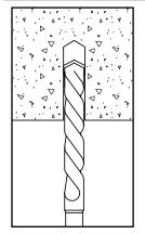
1.) Using the proper drill bit size, drill a hole into the vase material to the required depth.
