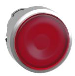
Head for illuminated push button, Harmony XB4, metal, red flush, 22mm, universal LED, spring return, for insertion legend
