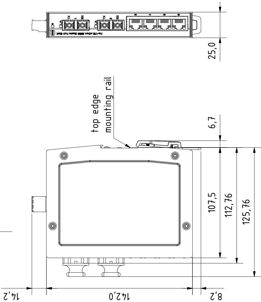
for mounting rail acc.to DIN EN 60715
