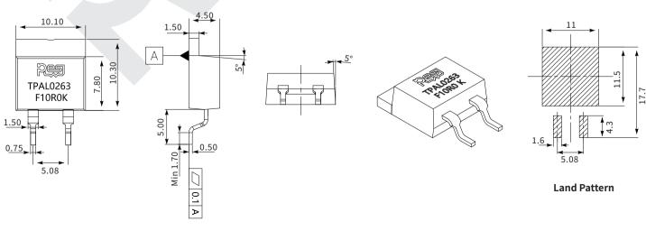
Note: The above dimensional tolerance is  $\pm$  0.3 mm.
