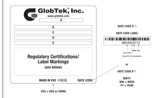
A=ICT / ITE / Medical Power Supply B=P/N: (料号) GTM91110P15024FSIM(R C=Model (型号) GTM91110P24024-F-S D=Input (输入)100-240V~, 50-60 Hz, 4.0A E=Output (输出)24.0 V == 6.25 A, 150.00W
