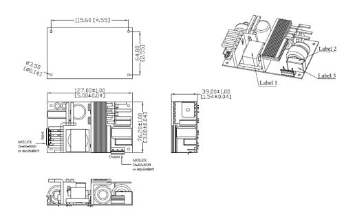
Label 1 Position Label 1 on top of Transformer
