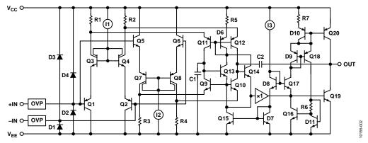
Figure 2. ADA4096-2 Simplfied Schemactic
