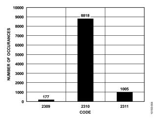
Figure 4. Histogram of Codes for 10,000 Samples Before Power Down
