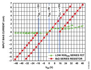
Figure 3. Input Current Limiting Capability
