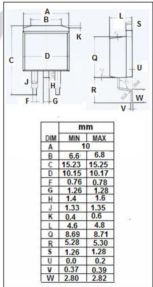
**isc N-Channel MOSFET Transistor****IXTA75N10P****• ELECTRICAL CHARACTERISTICS (T<sub>c</sub>=25°C)**
