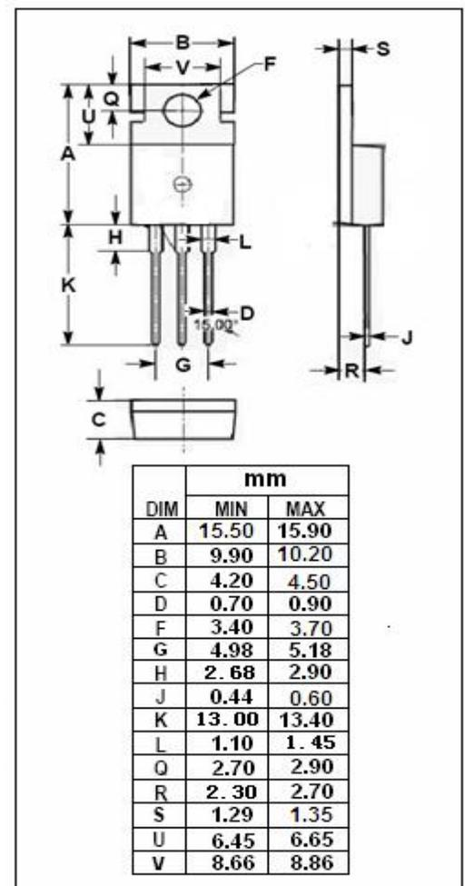
**isc N-Channel MOSFET Transistor      TK58E06N1, ITK58E06N1****ELECTRICAL CHARACTERISTICS**T<sub>C</sub>=25°C unless otherwise specified
