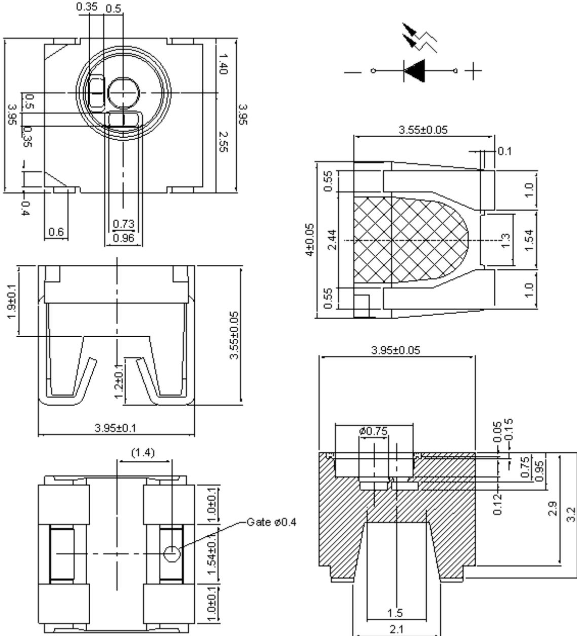
**Note:** The tolerances unless mentioned is  $\pm 0.1\text{mm}$  ,Unit = mm
