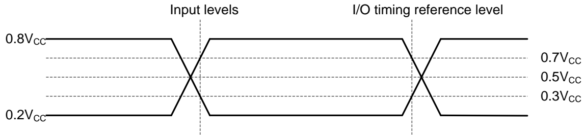
Figure 30: AC Measurement IO Waveform
